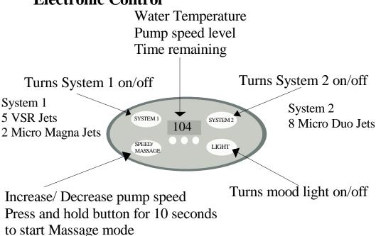
**System 1 Key:** Depressing the **ON/OFF** key will activate the jet pump at the highest speed level provided there is sufficient water in the tub or a jumper is inserted into the water level sensor input. The pump will remain ON for maximum time of 20 minutes of operation, after which it will automatically shut off. If the jet pump is already ON, depressing the **ON/OFF** key again will turn the pump OFF.
